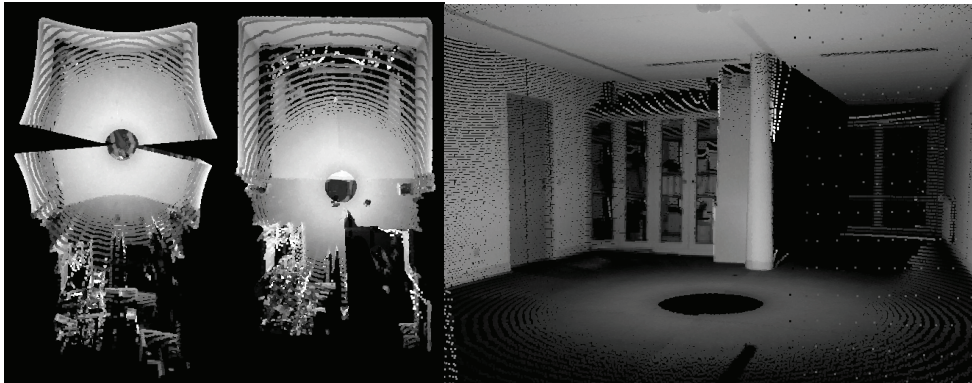
Fig. 3. a) Scan results without and with pose correction. b) 3D scan with remission values.
